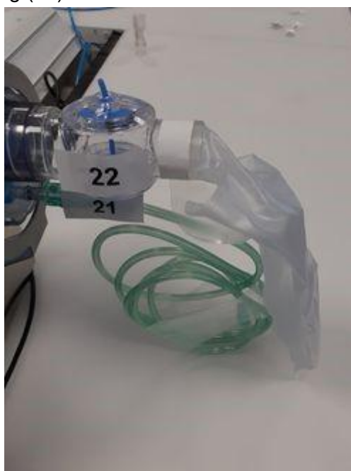
Figure 16: Connection of the tank to the AMBU balloon.
