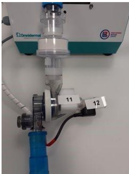
Figure 11: Connection of flow and pressure sensors.
