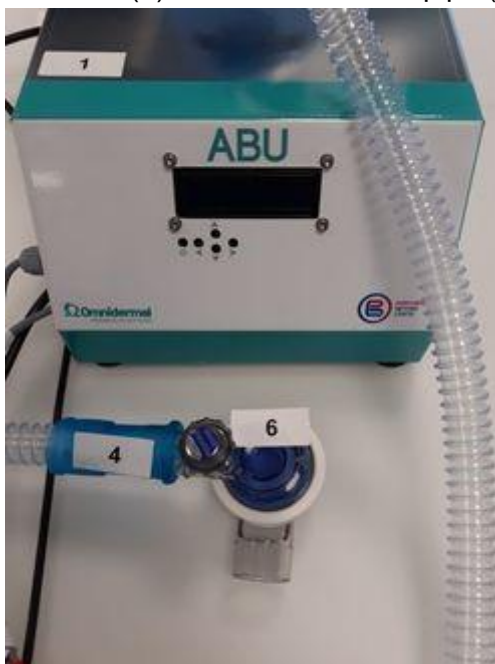
Fig. 8: Connection of the non-return valve to the air hose.
