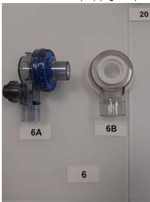
Fig. 9: Connection of the non-return valve to PEEP.
