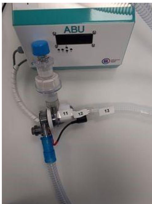
Figure 12: Connection of the sensors with the air hose.
