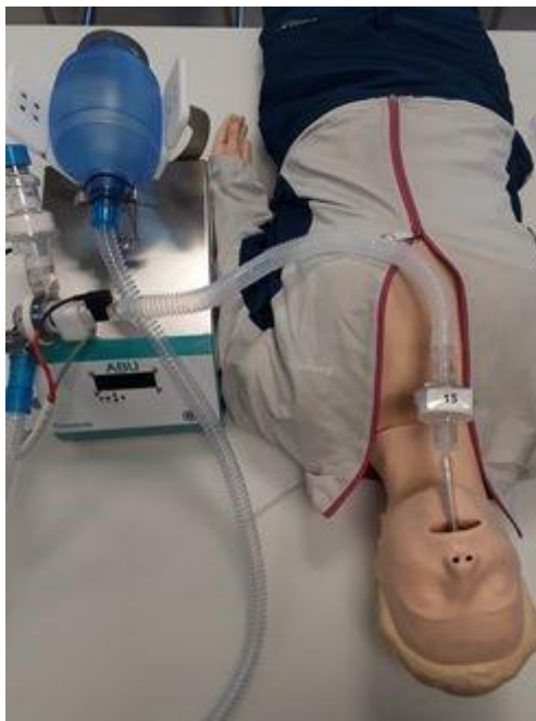
Figure 14: Connection of the system to the endotracheal tube.
