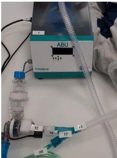
Figure 23: Connection of the adjustable air hose to the Y-connector.
