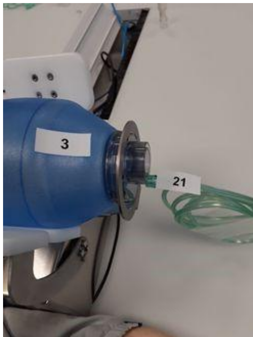
Figure 15: Connection of the oxygen tube to the AMBU balloon.
