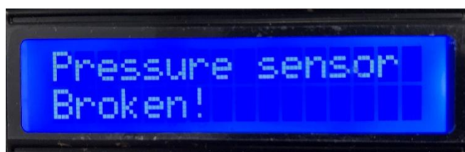
Figure 49: Faulty differential pressure sensor alarm screen
