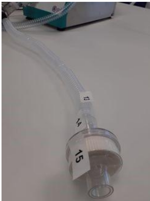
Figure 13: Connection of the filter to the adjustable air hose.
