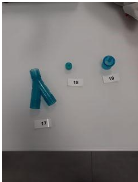
Figure 17: Y-connector and its parts.
