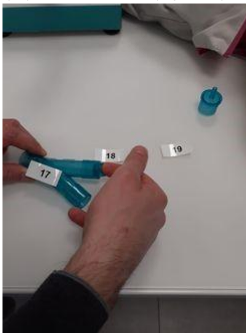
Figure 19: Method for inserting the one-sided valve.
